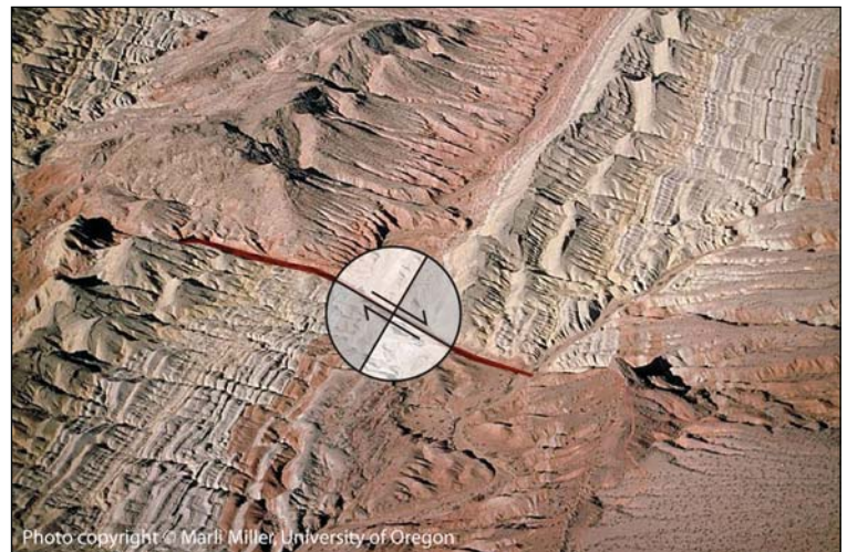
Figure 3. A first-motion diagram for an earthquake along the San Andreas Fault shows an alternating black and white pattern. White areas represent where P waves begin as dilatations and black areas represent where P waves begin as compressions.
