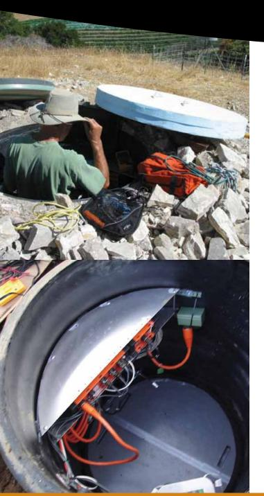
deployed from west to east on a regular grid with 70-km (42-mi) spacing. Each station records ground motion for about two years before it is dismantled and the equipment is reinstalled at another location on the eastern edge of the array. When completed, this program will have occupied over 1600 locations in the conterminous United States.
