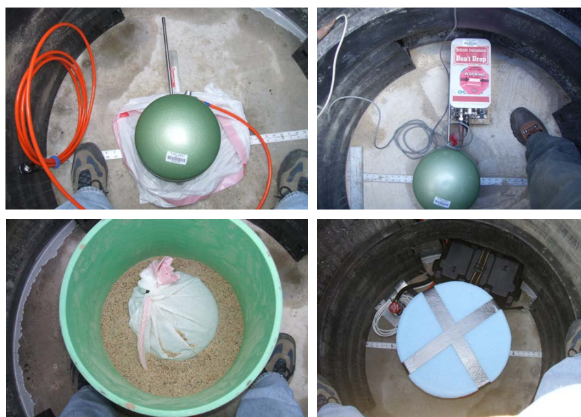
Figure 2-24. Orientation of an STS-2 seismometer at TA.N15A using the Octans. Notice the shock watch stickers that might indicate an Octans had suffered a crippling impact. Once oriented, the sensor is then packaged and insulated.
